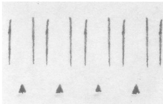
FIG. 12— Royal 5000 series hammer marks. The triangular images below the marks are caused by a remnant of the spoke.
